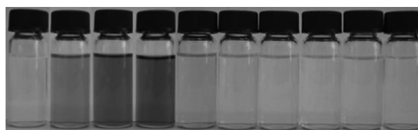
Figure 4. Color changes observed on 1 (25 μM) in the presence of metal ions in CH 3 CN/H 2 O (95:5). From left to right: no ion, Cd 2+ , Ni 2+ , Cu 2+ , Pb 2+ , Ag + , Na + , Mg 2+ , Hg 2+ , and Zn 2+ (20 equiv.). The color version is shown in Figure S2, in the Supporting Information.
